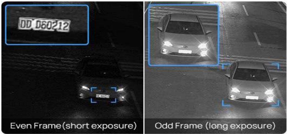
FIGURE 3: Comparison between short-exposure and long-exposure frames for improved nighttime license plate detection.
