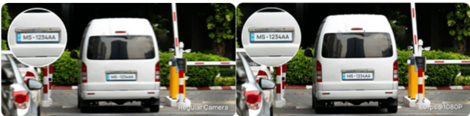
FIGURE 5: Improvement in plate-recognition accuracy using a 60 fps @1080p camera compared to a regular imaging sensor.
