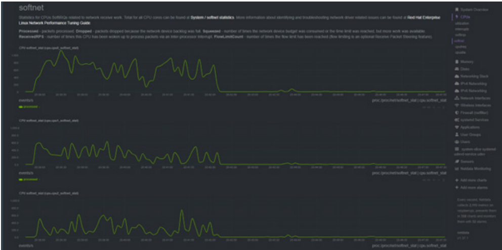
FIGURE 4: Softnet Statistics During DDoS Simulation
