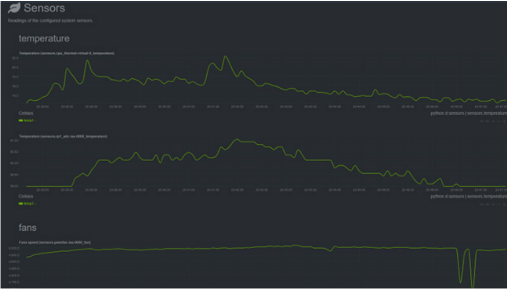
FIGURE 8: System Temperature and Fan Speed During DDoS Simulation
