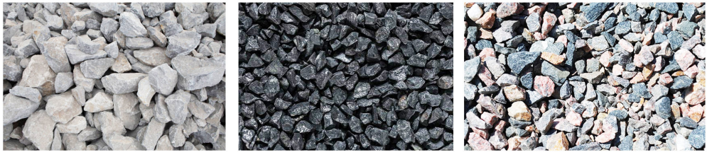
FIGURE 4. Aggregates of different rocks. Limestone (a), basalt (b), granite (c)
