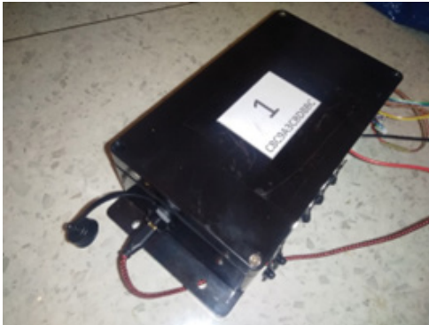
FIG. 18. – Some devices “IoT for structure” made by the authors, in the research team “Moni2BSafe” at University of Rome “Tor Vergata”. It is visible the hexadecimal number, meaning the wifi tag of the device.
